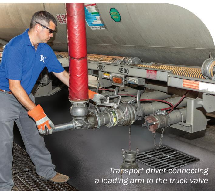
Transport driver connecting a loading arm to the truck valve
